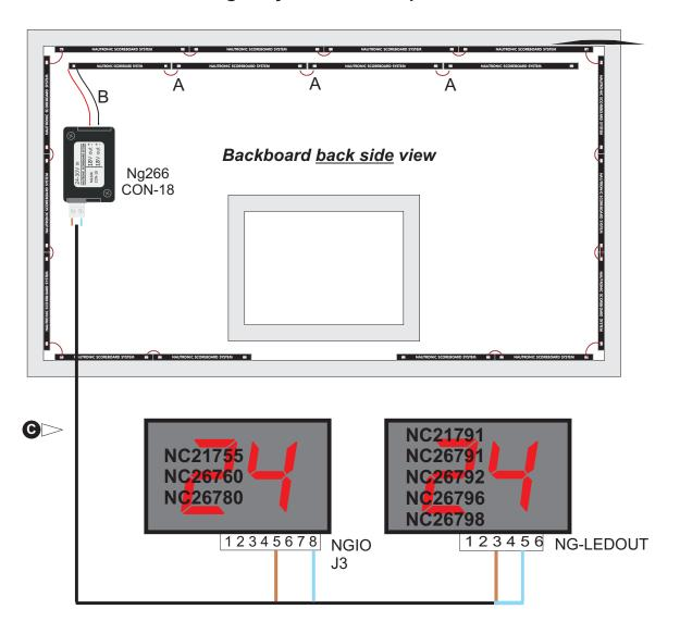
Connect "+" to "+" using red wire and "-" to "-" using black wire.
